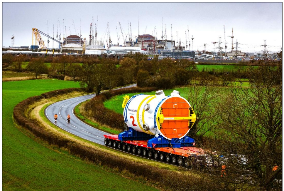
The second nuclear reactor approaching Hinkley Point C. The domes of on the two new reactor buildings are in the background. Image: EDFenergy
