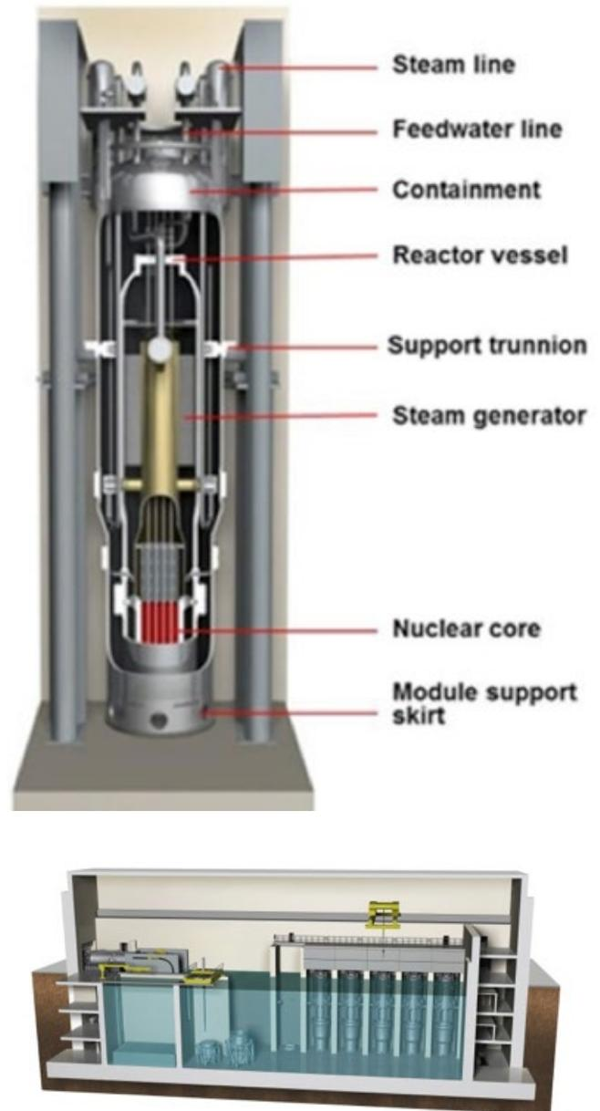
**NuScale Power Module (US NRC) [top panel] and reactor building [bottom panel]. (Images courtesy of NuScale Power)**
