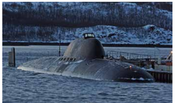
The Russian Alfa-class submarine which used a lead-bismuth fast reactor. It could run at up to 41 knots.
